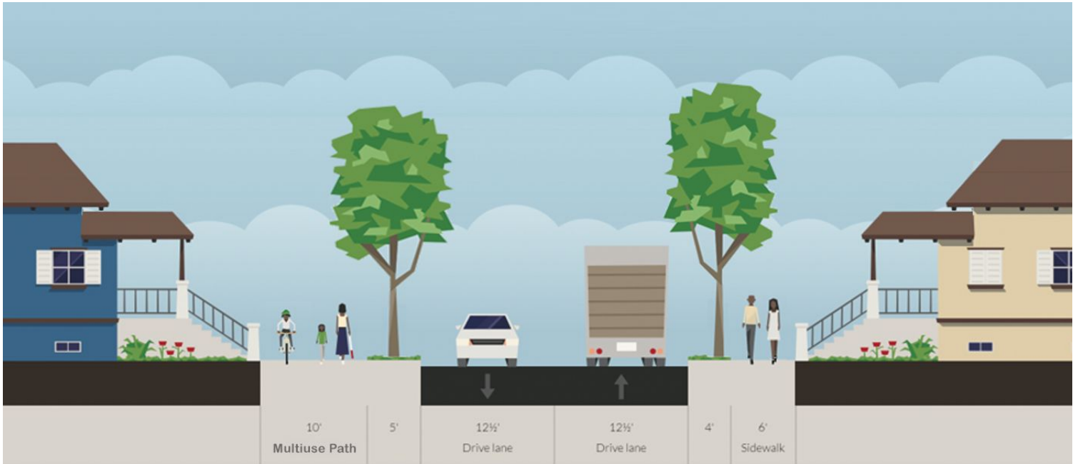
Proposed 10' multiuse protected pathway on the south side of Glenwood Ave. Pedestrian-only sidewalk on the north side.
